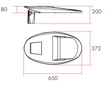
Adjustable luminaire tilt in top and side mounting
